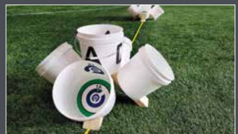
With some lumber, five-gallon buckets and basic hardware, NIST apparatus like this makes it possible to establish a benchmark for drone pilot skills that can be compared worldwide and through time.
