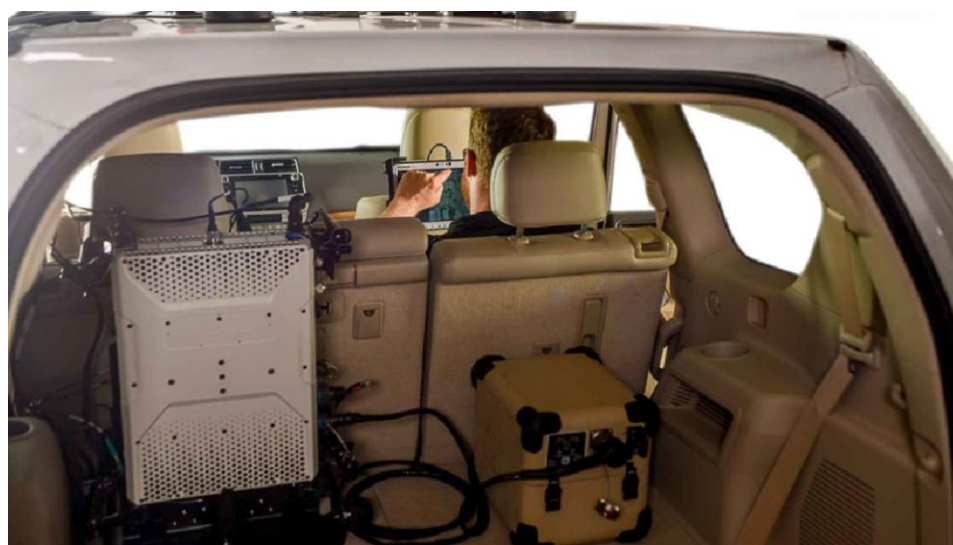
EnforceAir2 installed in a vehicle
